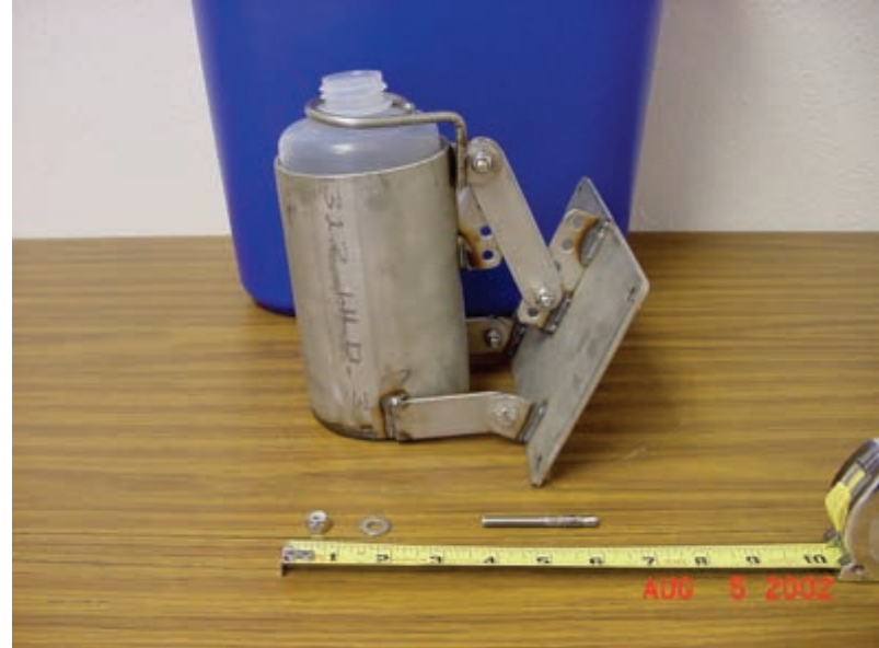
Figure B2-21 Stormwater Sediment Traps
