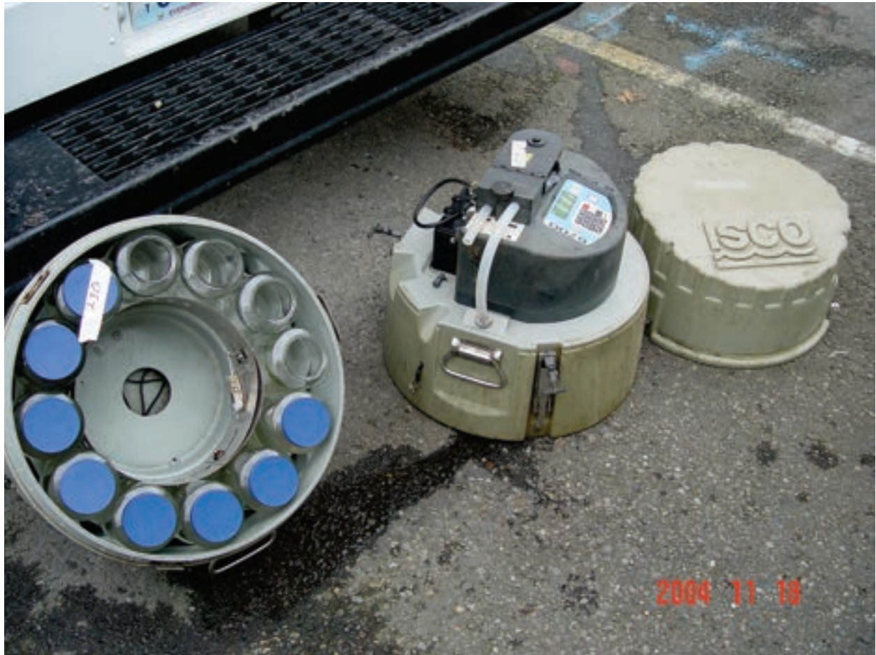
Figure B2-20 Sequential Sampler Base
